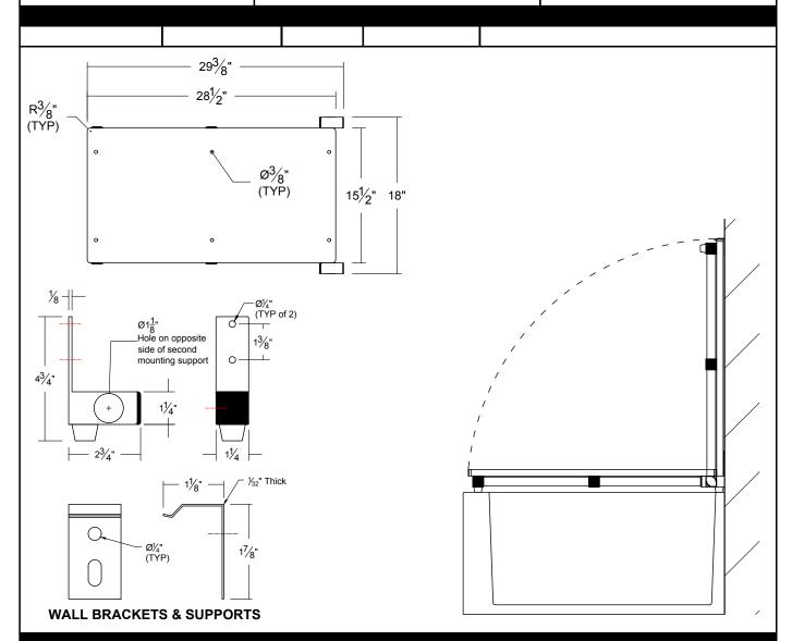
Seat: Fabricated of  $\frac{3}{4}$ " solid one piece, white HDP (High Density Plastic) with radius leading edges to prevent injury. Secured to frame by means of  $\frac{1}{4}$ " stainless steel rivets. Seat material is warp / water resistant and will not support bacteria or fungi. There are no chemicals that may irritate human skin.
